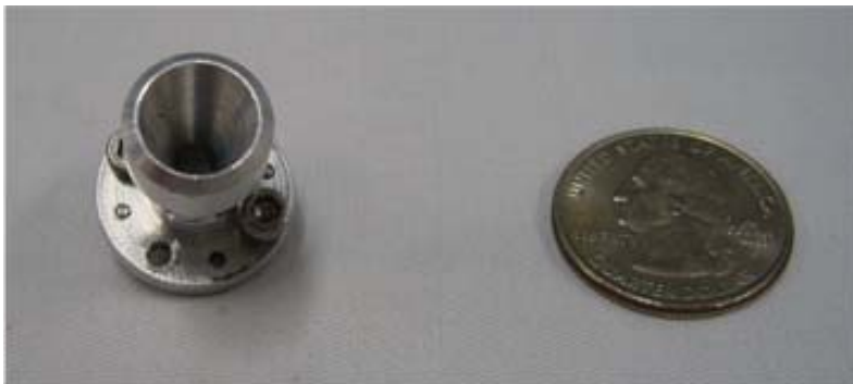
Conical horn antenna Beam-width 30 deg
