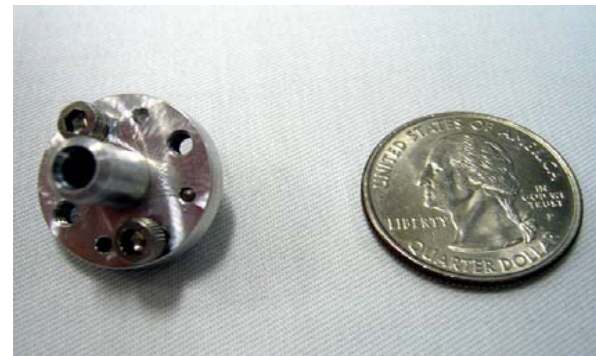
Conical horn antenna Beam-width 60 deg
