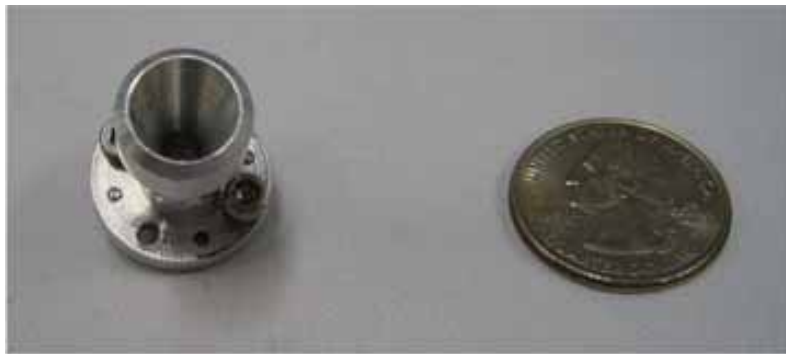
Conical horn antenna Beam-width 30 deg
