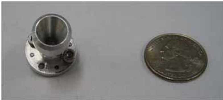
Conical horn antenna Beam-width 30 deg
