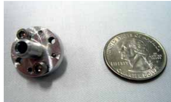
Conical horn antenna Beam-width 60 deg
