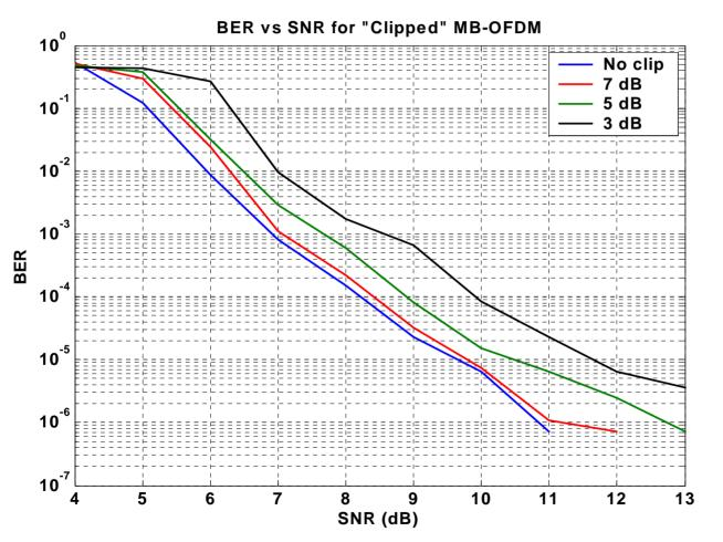
Simulation 480 Mbps DCM 3⁄4 Rate Coding AWGN only
