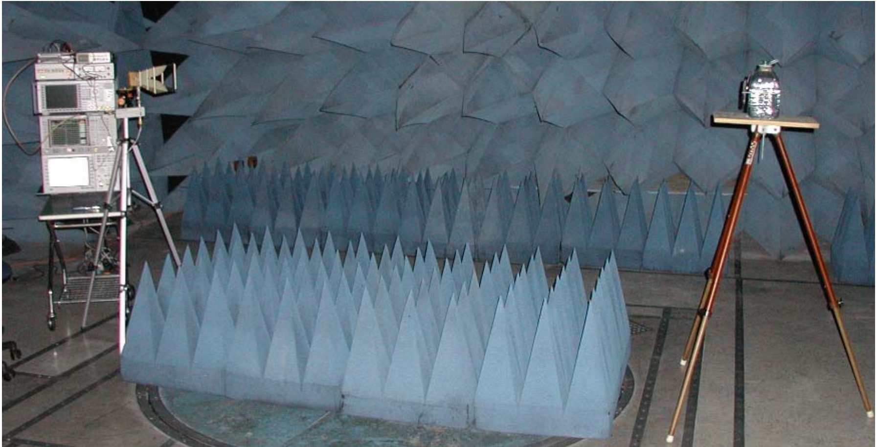
Figure 2c – Free space test configuration in the shielded FAU EMI anechoic chamber.
