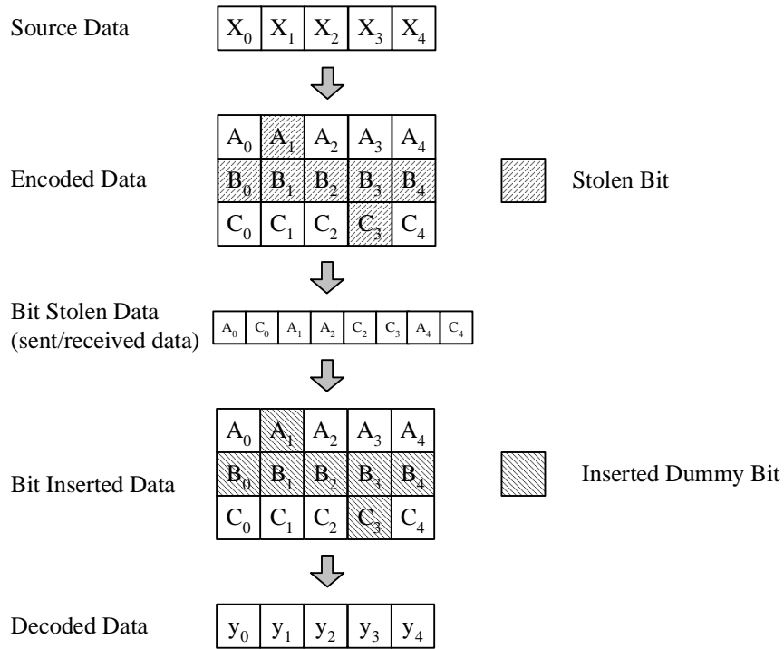
Figure 15—An example of the bit stealing and bit insertion procedure ( R=5/8 )
