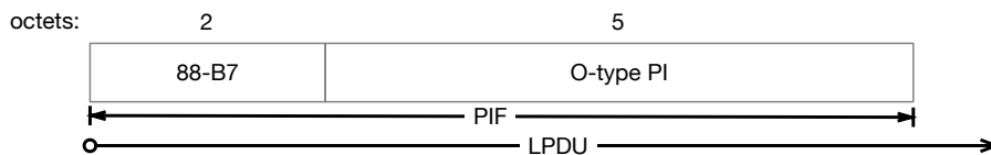
Figure LT-OE— Type 3 PIF encoding of an O-Type protocol identifier
