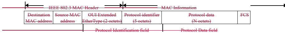
Figure 16—IEEE 802.3 frame with the OUI Extended EtherType encoded in the Length/Type field
