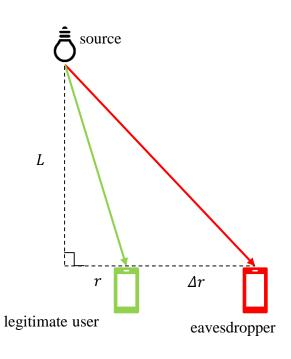
Simulation parameters: transmit power 1 W; Lambertian order 1; L=2.15 m; PD area 1 cm^2; PD responsivity 0.4 A/W.
