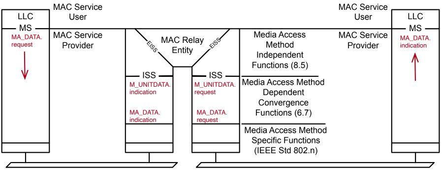
NOTE-The notation IEEE Std 802.n in this figure indicates that the specifications for these functions can be found in the relevant standard for the media access method concerned; for example, n would be 3 (IEEE Std 802.3) in the case of Ethernet.
