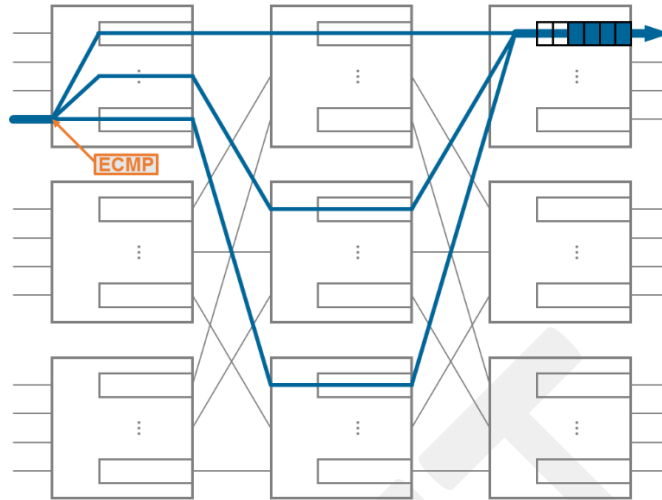
Figure 7 – ECMP Load Balancing
