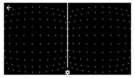
This can save some direct computation and let the GPU do a fair amount of interpolation. Rather than having to apply to every single pixel (1920 \* 1080 ~= 2e6), we do the calculation for every vertex in the mesh (40 \* 20 = 800). The result is a significant reduction (3 magnitudes or so) of computation, and a nice boost in performance. The WebVR Polyfill currently implements this approach.
