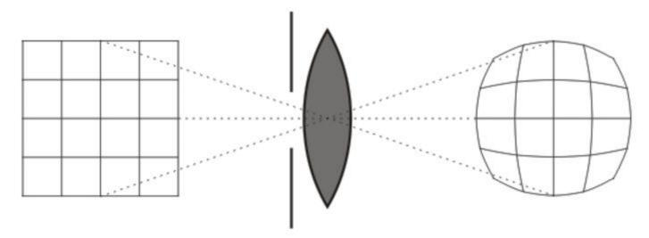
Lens distortion is well understood mathematically, governed by equations like these, with distortion coefficients corresponding to the particular lens. To undo the distortion properly, we also need to calculate the centers of the eyes, which requires knowing a bit about the geometry of the display and the enclosure itself. This can all be done, even on the web! I summarize a few implementation options below.
