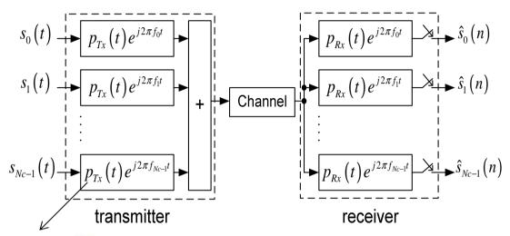
prototype filter: Typically  $KN_c \pm 1$  samples long.
