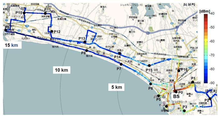
•Site measurement of received power vs. distance with base station antenna height: 45m
