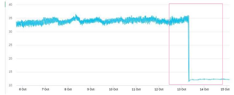
A gradual increase in belt frequency was observed for 5 to 6 days and showed a transition in an exponential trend before the failure.
