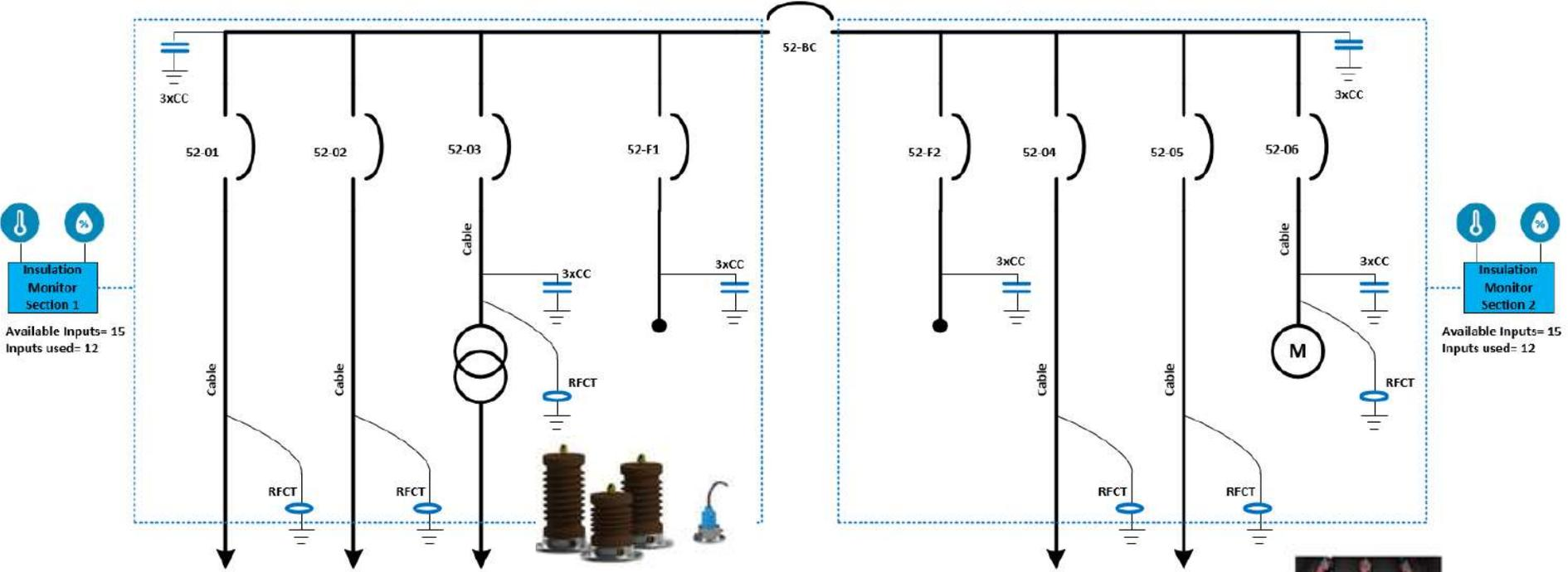
Protected assets: 2 semi-bars, transformer, motor, 6 cables, 9 CB
