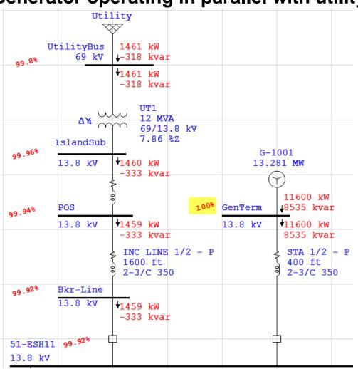
With the utility transformer tapped at nominal and the generator AVR in voltage control at 100% there is an export of 333 kvar, a leading PF of 97.5%
