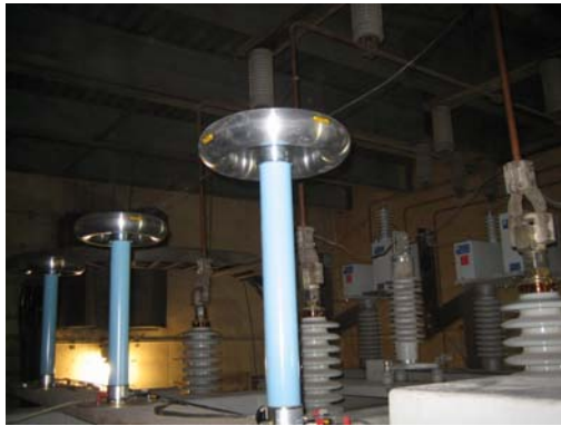
Voltage Dividers Installed at Primary Bushings of Transformer
