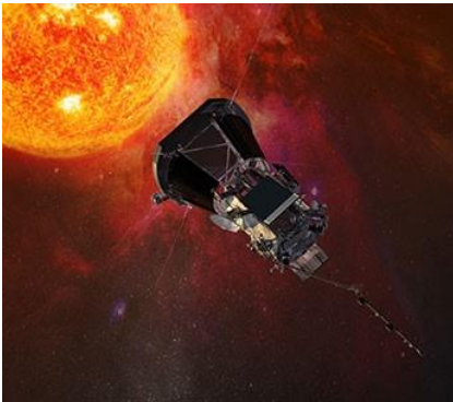
The solar panels are shown here on this artist rendering of Parker Solar Probe; they are the black squares with gray rectangles on the center of the spacecraft. Credit: NASA/JHUAPL
