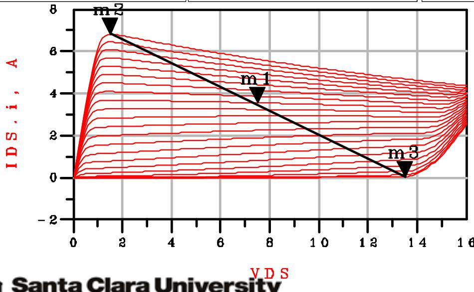
10W design ;  $V_{m2}=1.5V$
