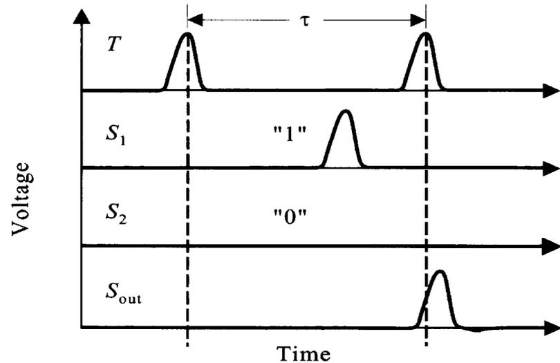
**Picosecond-scale pulses with amplitude less than 1 mV carry data between gates. Clock and data pulses are same.**
