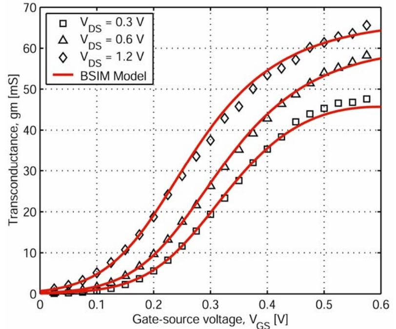
Measured and modeled  $g_m$  vs.  $V_{GS}$ .
