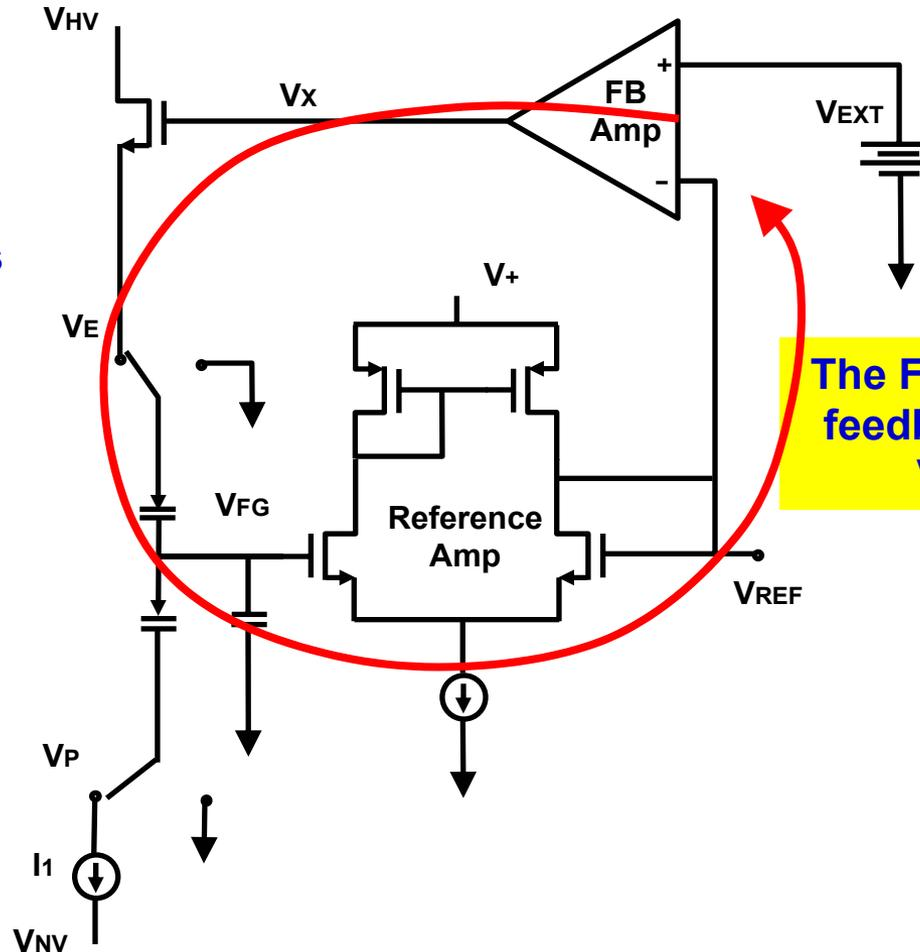
The FB Amp drives the feedback loop so that  $V_{REF} = V_{EXT}$
