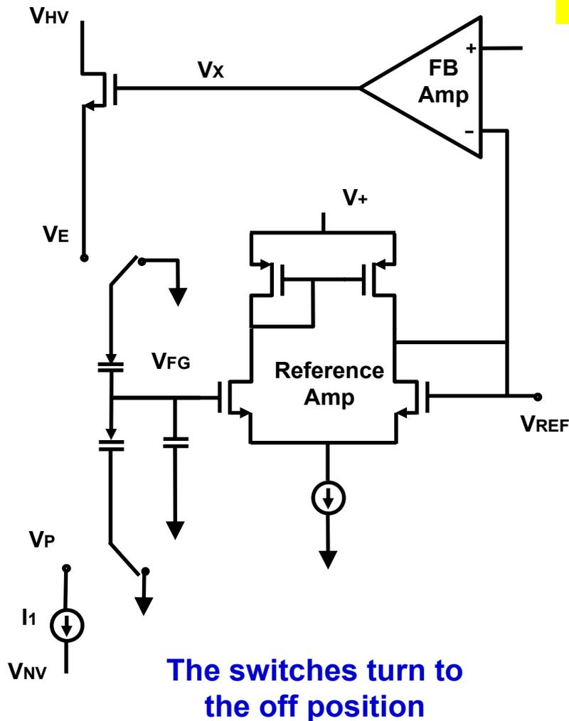
The external reference voltage is disconnected
