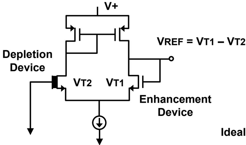
$$V_{T1} = \frac{Q_E}{C_{gate}} + V_{T0}$$
