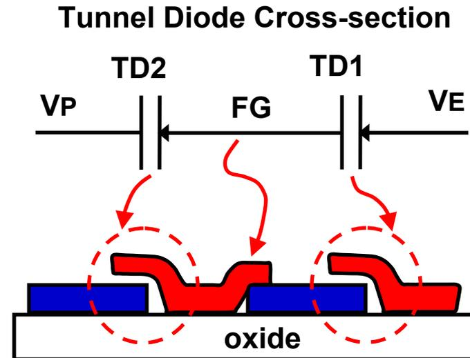
**FG is isolated by oxide and cannot gain or lose charge under normal conditions**
