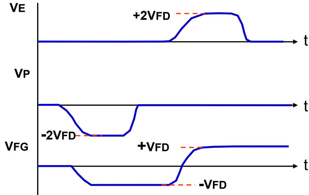
**Voltage swing on FG conceptually  $2V_{FD}$  (= 24V for 12V  $V_{FD}$ )**
