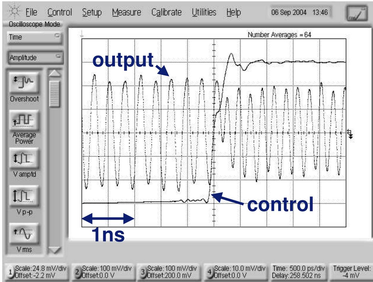
Calculate FFT to measure the switching time
