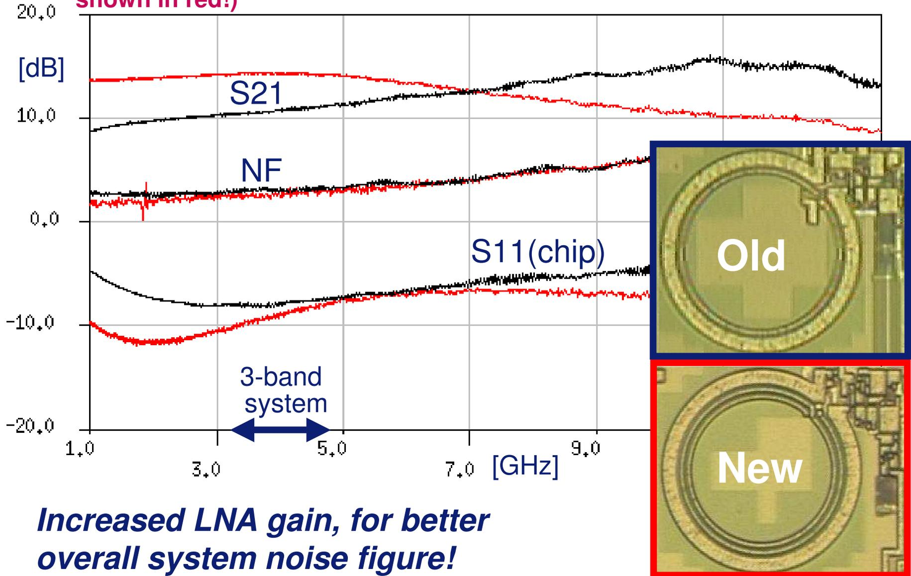
**Increased LNA gain, for better overall system noise figure!**
