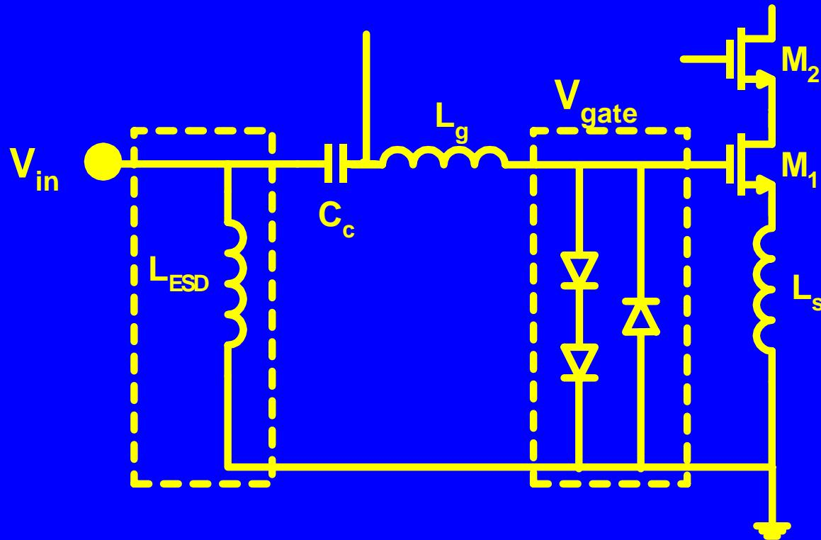
Schematic with additional diodes
