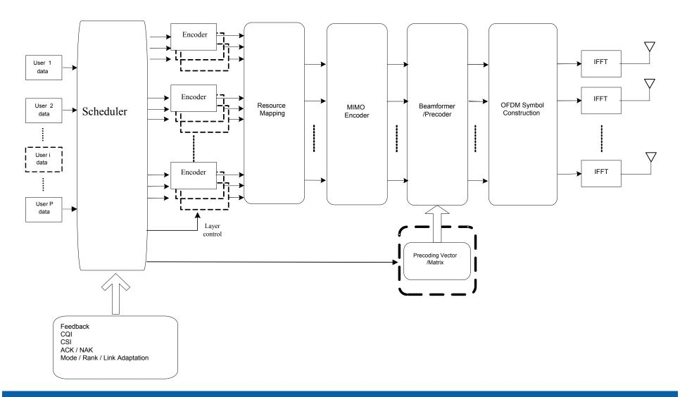
•Figure extracted from IEEE 802.16 reference 8 •Vertical Encoding requires a single Encoder Mobile Wireless Group
