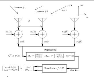
$$m{r}(k) := \sum_{l=0}^{J} lpha_l b_l(k) m{s}_l + m{n}(k), \; orall k \geq 0, \qquad m{s}_l : ext{Steering vectors}.$$
