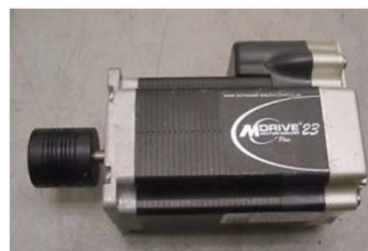
Stepping motor with integrated controller (uses programmable firmware)
