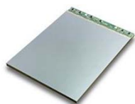
Dexela 2329 .075 mm pixels 26 FPS / CMOS 70 FPS @ 2x2
