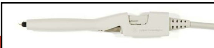
12 GHz Differential Browser: 210 fF input C, 50 kOhm input R, 0.2-3.3 mm lead span
