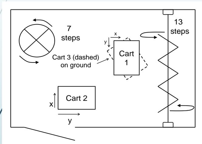
Measure effects of paddle angle and antenna position at three locations in a loaded chamber
