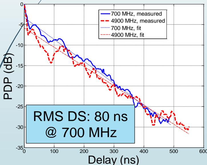
Reverberation chamber can easily replicate diffuse multipath
