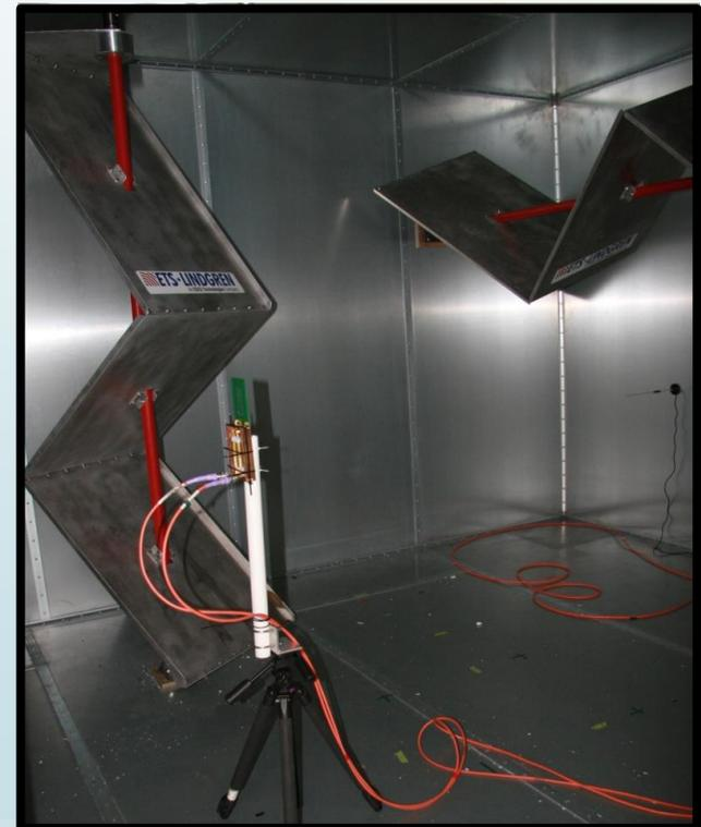
NIST measurements of prototype 4G MIMO cellular telephone antennas
