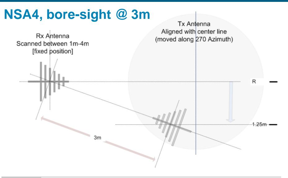
**Single Point** In order to verify NSA3, a measurement was repeated at 3m distance with the tx antenna, taking a 1.25m offset from the center line.
