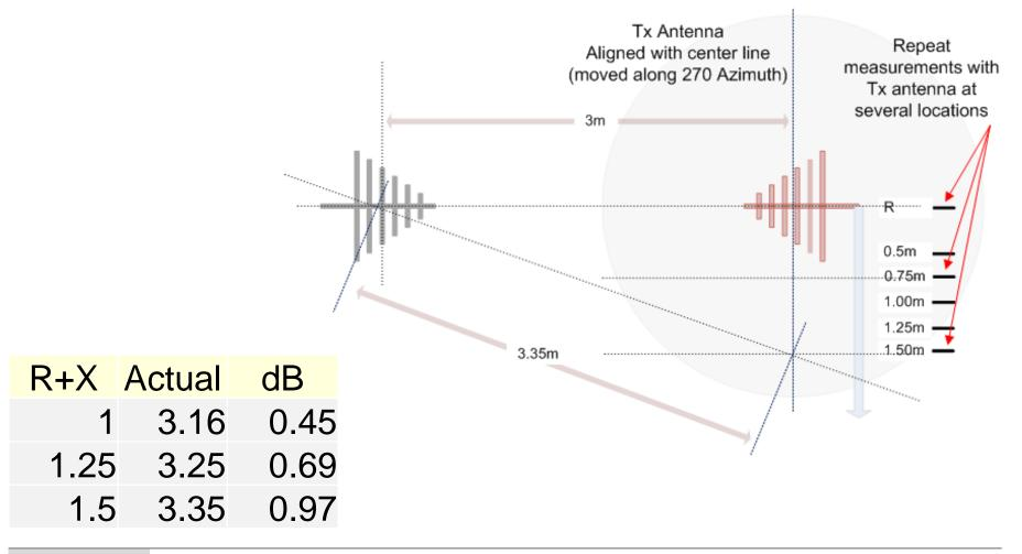
Meas Dist Error with NSA1 & NSA2, comparing response with 3m limits but the measurement distance is increased. Hence results need offsetting by 20 Log (actual distance / 3)
