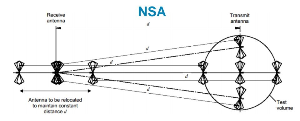
AlignmentIt is clear from the wider positions that both the Tx/Rx<br/>antennas are aligned.AlignmentTo get an improved verification the alignment of the rx<br/>antenna should not be changed. In addition, the actual<br/>position of the Rx antenna should not change either<br/>because during the test, the antenna is not moved.
