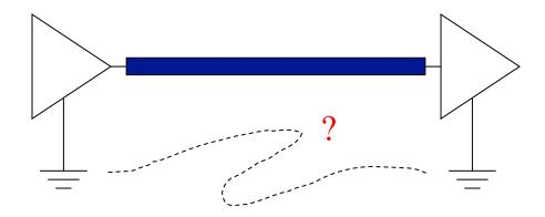
• Is ground a zero-impedance equipotential surface?
