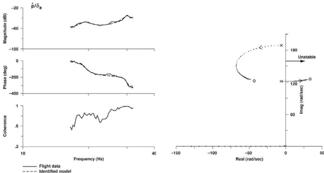
$$\frac{p}{\delta_a} = \frac{L_{\delta_a}}{(s - L_p)} + \frac{K_1 s}{[s^2 + 2\zeta_1 \omega_{n_1} s + \omega_{n_1}^2]} + \frac{K_2 s}{[s^2 + 2\zeta_2 \omega_{n_2} s + \omega_{n_2}^2]} + \dots$$
