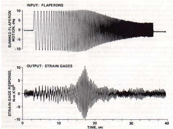
Fig. 5 Input and output time histories for one symmetric flaperon sweep (beam mode).
