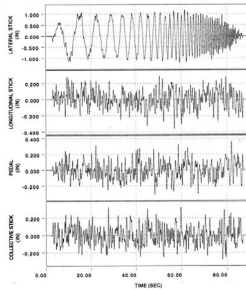
Figure 3: Feedback loops to maintain attitude during frequency sweep
