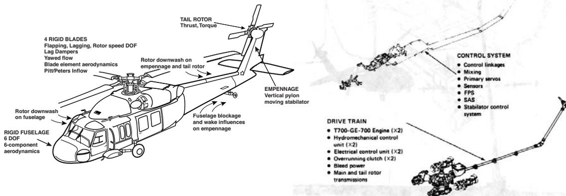
Fig. 1. Sikorsky-Ames Gen Hel UH-60 real-time simulation model.
