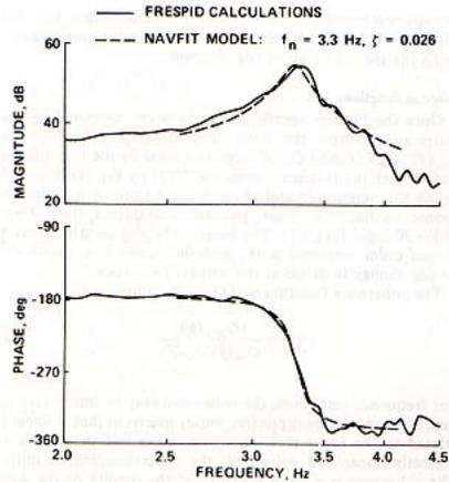
Fig. 6 Symmetric beam mode frequency response and fitted second-order model.
