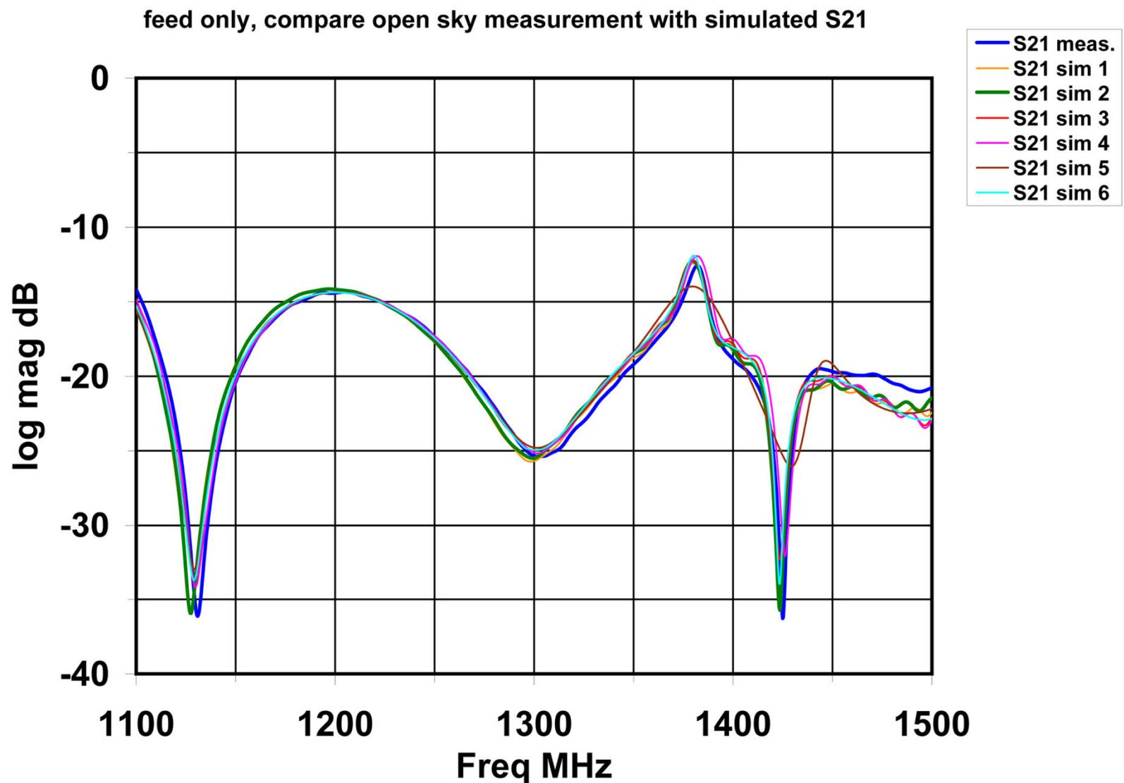
**Figure 7: Compare actual measurement data dB[s21] with the simulations**
