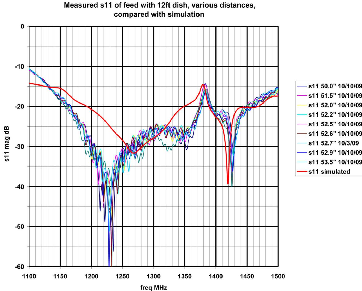
**Figure 25: Measured s22 of the feed with an actual 12 foot dish at various distances from the vertex, compared with simulation**
