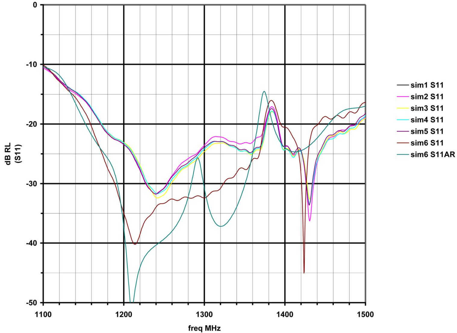
Figure 15: Compare four S11 simulations of the feed with 10 lambda dish
