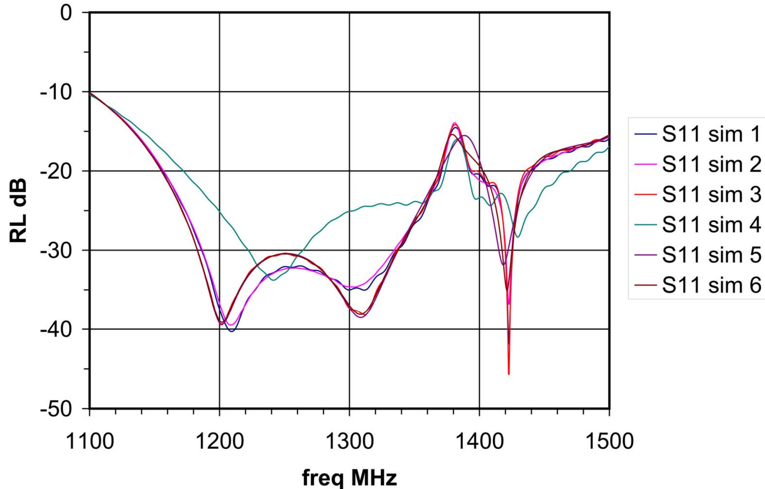
**Figure 10: Compare six simulations of the port s11**
