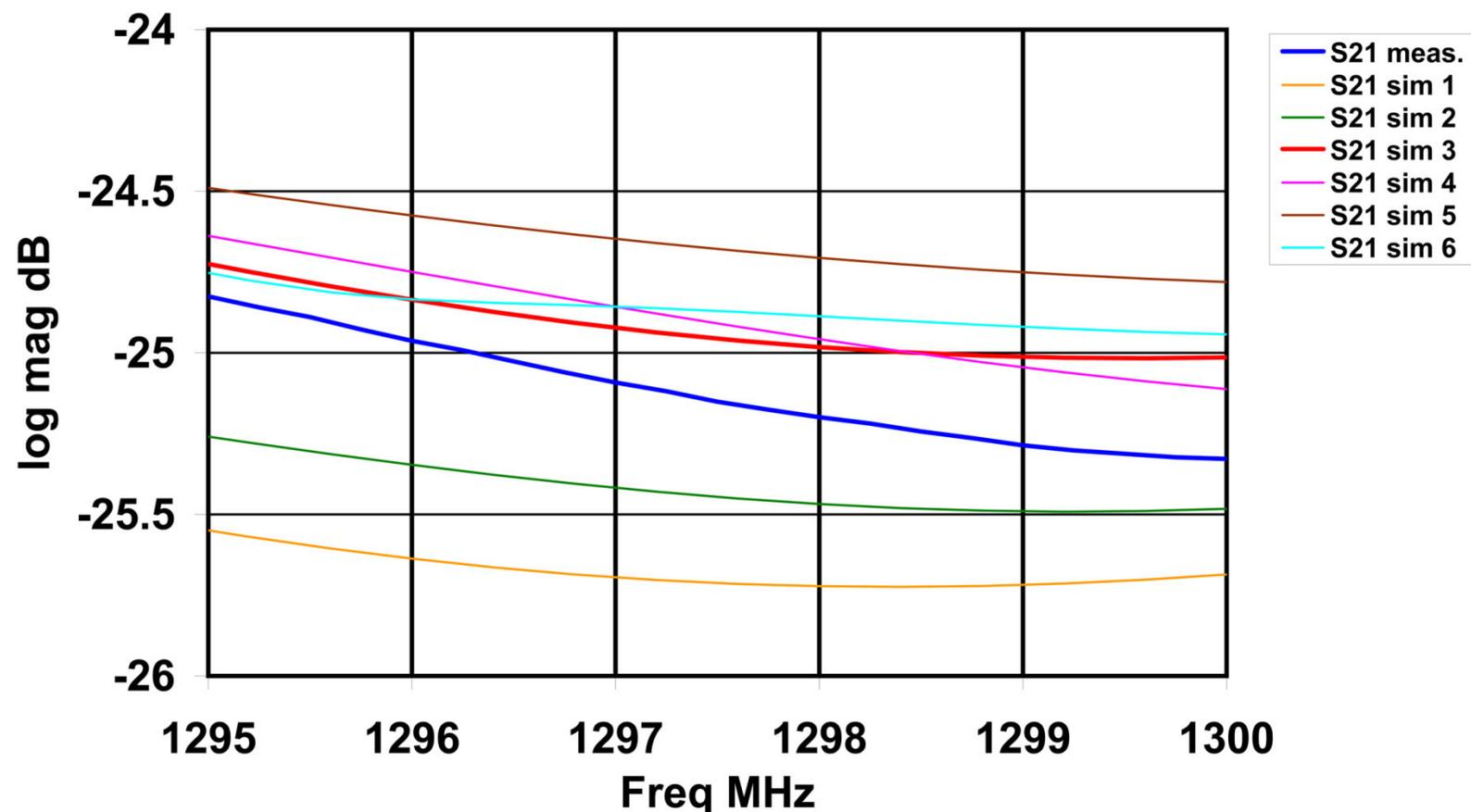
Figure 9: Compare actual measurement data with the simulations over the narrow frequency span of 1295MHz to 1300MHz
