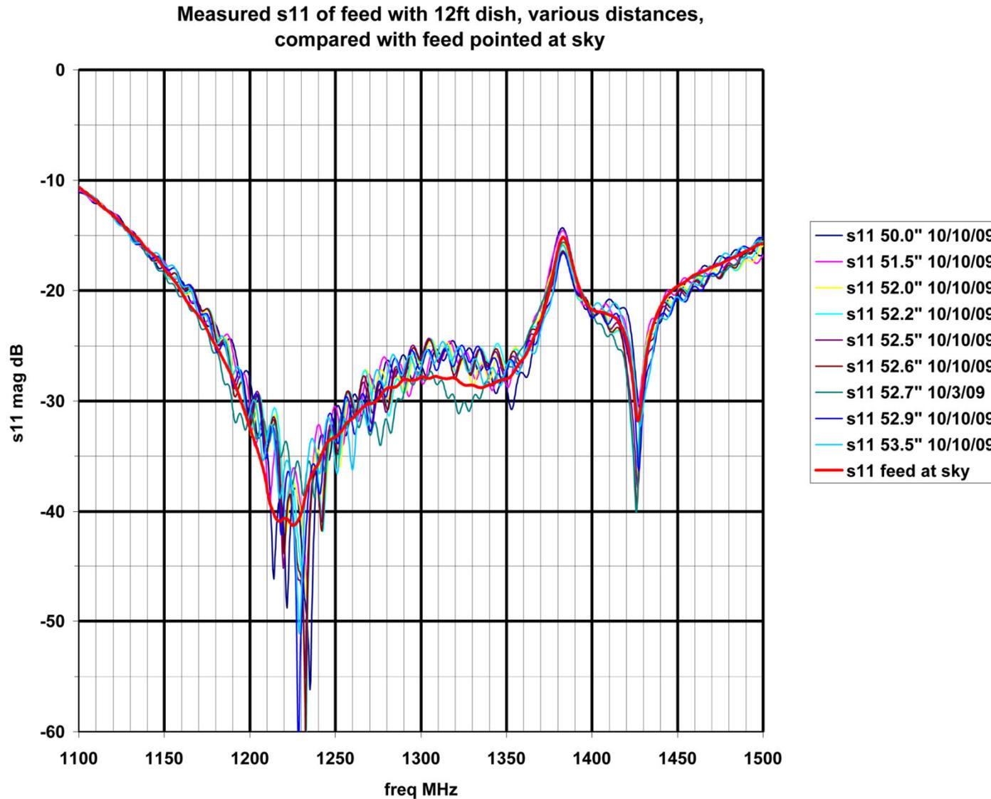
**Figure 27: Measured s22 of the feed with an actual 12 foot dish at various distances from the vertex, compared with measurement of the feed pointed at open sky**
