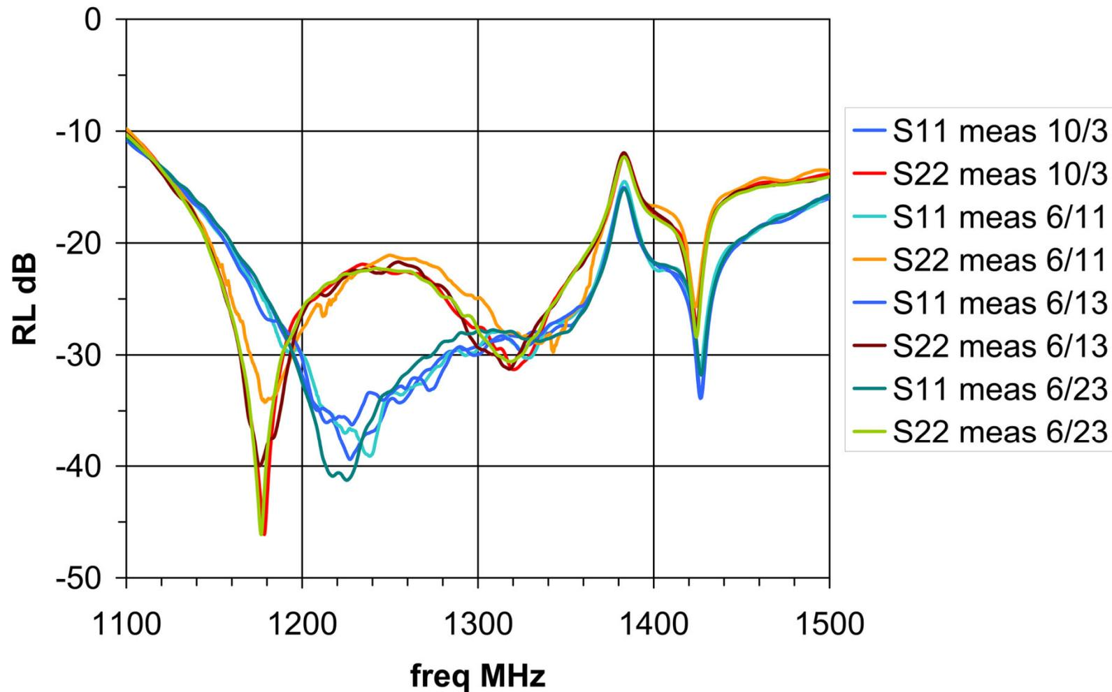
**Figure 11: Compare four different measurements of the actual feed**
