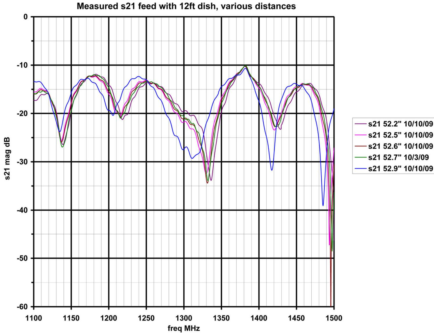
**Figure 29: Measured s21 of the feed with an actual 12 foot dish at various distances from the vertex, compared with the simulation**
