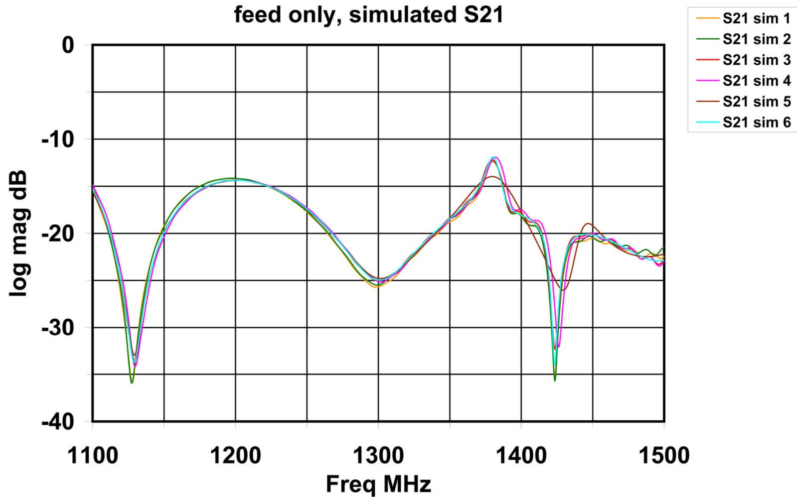
**Figure 6: Compare six s21 simulations of the feed**
