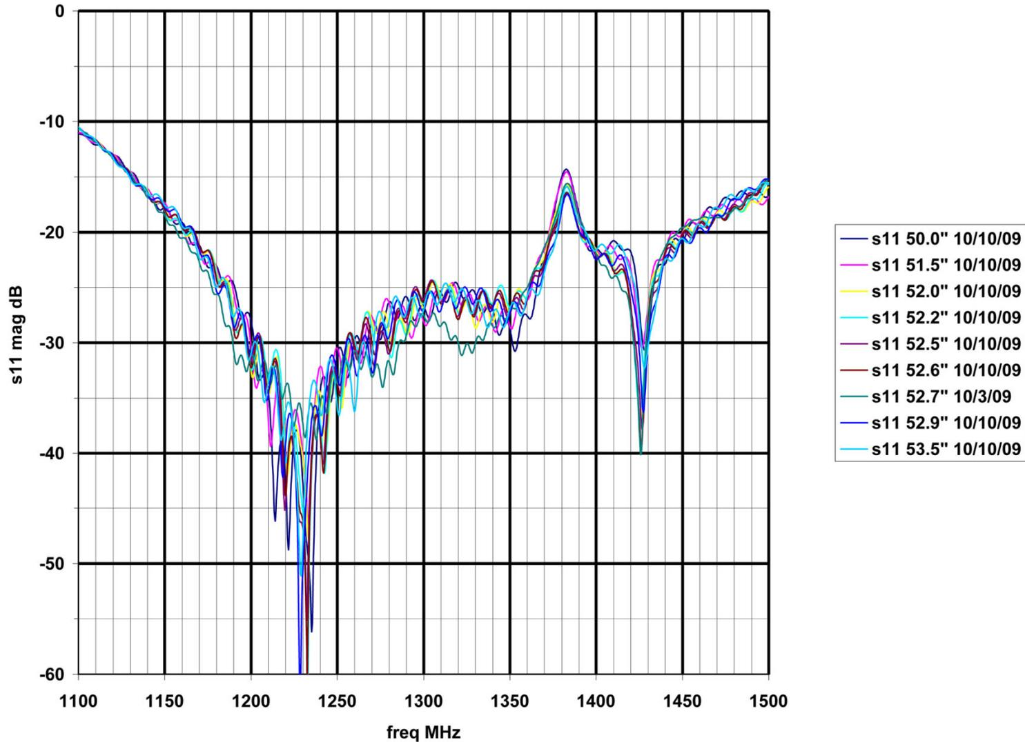
**Figure 23: Measured s22 of the feed with an actual 12 foot dish at various distances from the vertex**
