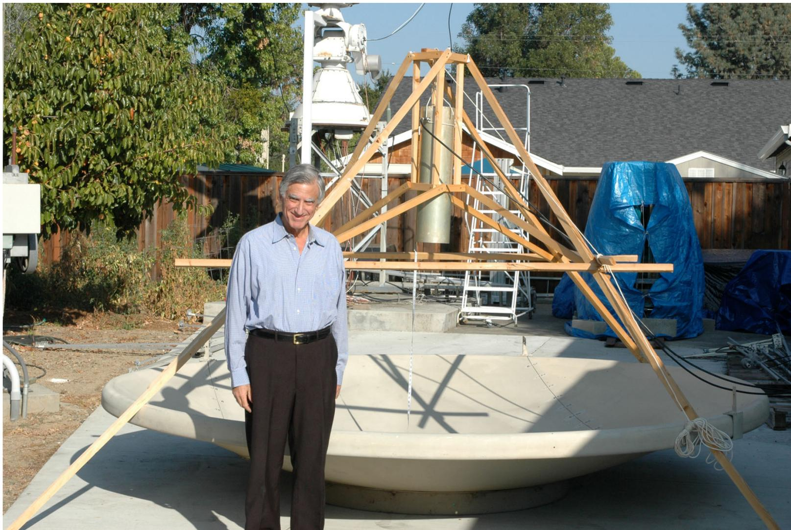
**Figure 21: Feed supported above the dish**
