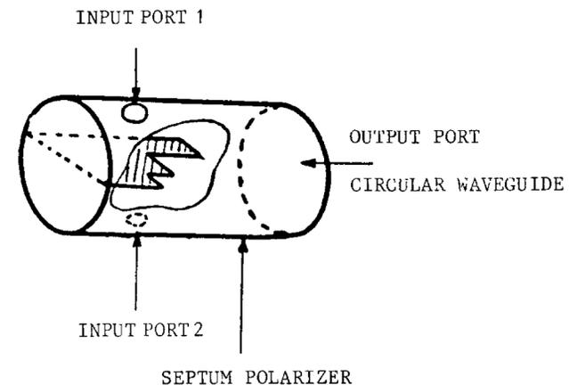
Fig. 1. Septum in circular waveguide.
