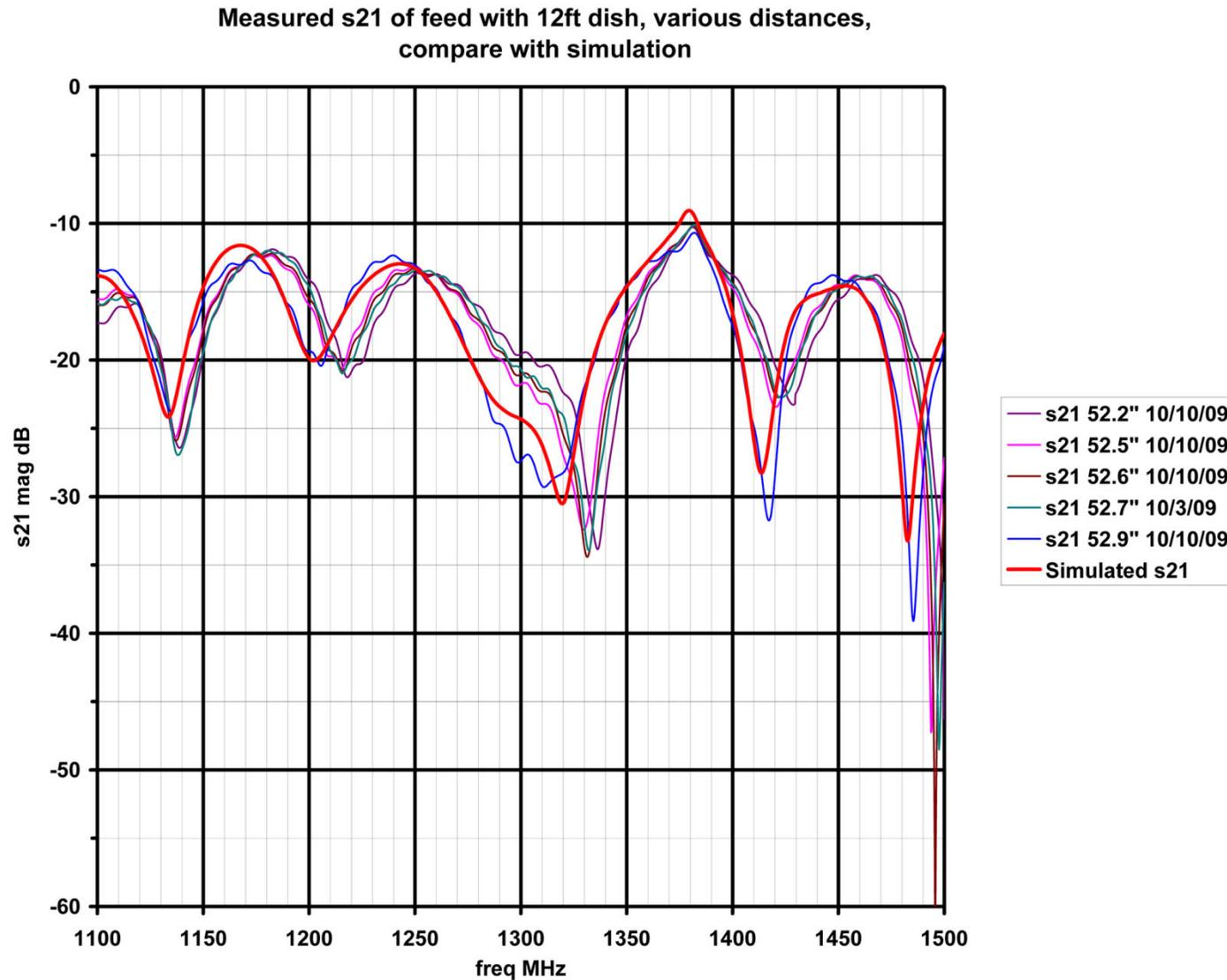
**Figure 30: Measured s21, compared with the simulation, narrow frequency range**
