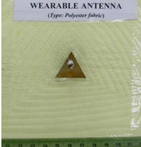
Fig. 2 Photograph of the fabricated wearable antenna
