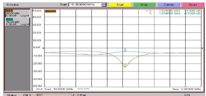
Figure 5(a). S21 vs Frequency
