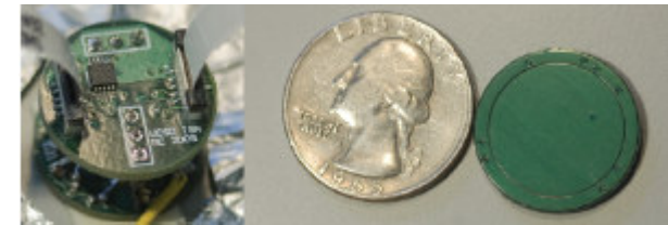
[Y. M. Chi, S. R. Deiss and G. Cauwenberghs, "Non-contact Low Power EEG/ECG Electrode for High Density Wearable Biopotential Sensor Network", 6th International Workshop on Wearable and Implantable Body Sensor Networks, 2009]
