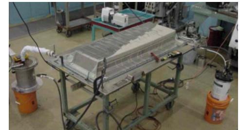
Resin Transfer Molding (RTM)
