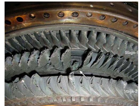
Nozzle guide vane burned out
