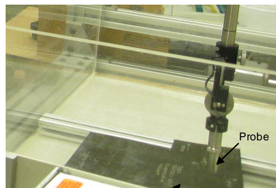
Water Immersion Ultrasound Scanning Tank
