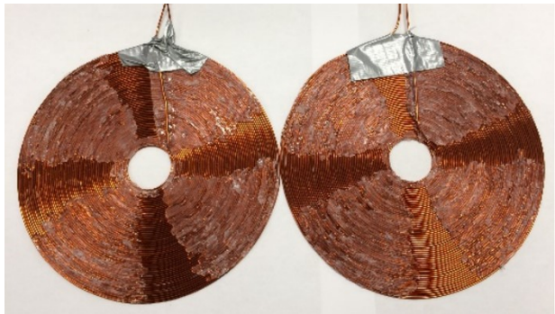
Flat coils used for data transfer
