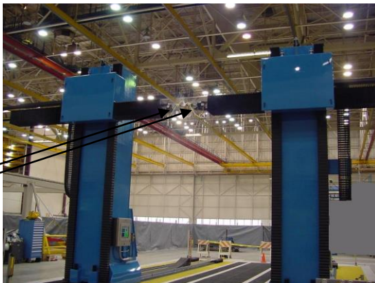
Large Thru Transmission Ultrasound Water Squirter System
