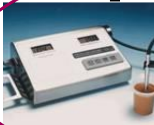
Cadburys ultrasonic chocolate particle sizer
