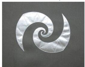
Fabric equiangular spiral antenna
