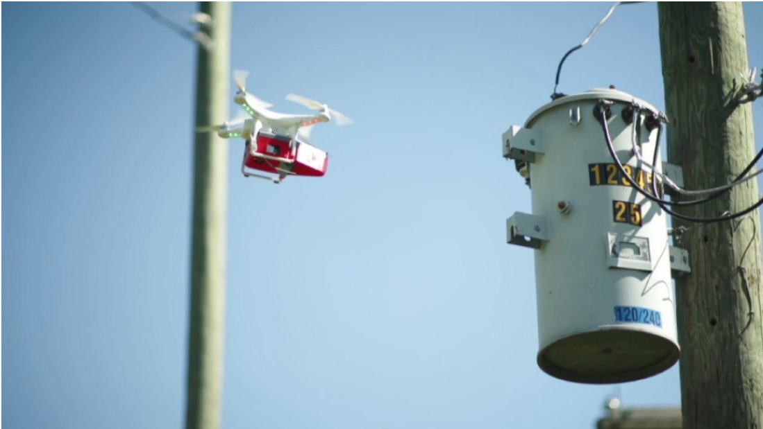
Drone monitoring a mounted transformer
