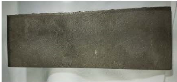
Titanium Grade-2 bar stock, 50mm x 150mm 6mm.
