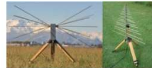
Fig. 2. (left) Biconical antenna PMM BC-01 and (right) log-periodic antenna PMM LP-02 on the measurement field.
