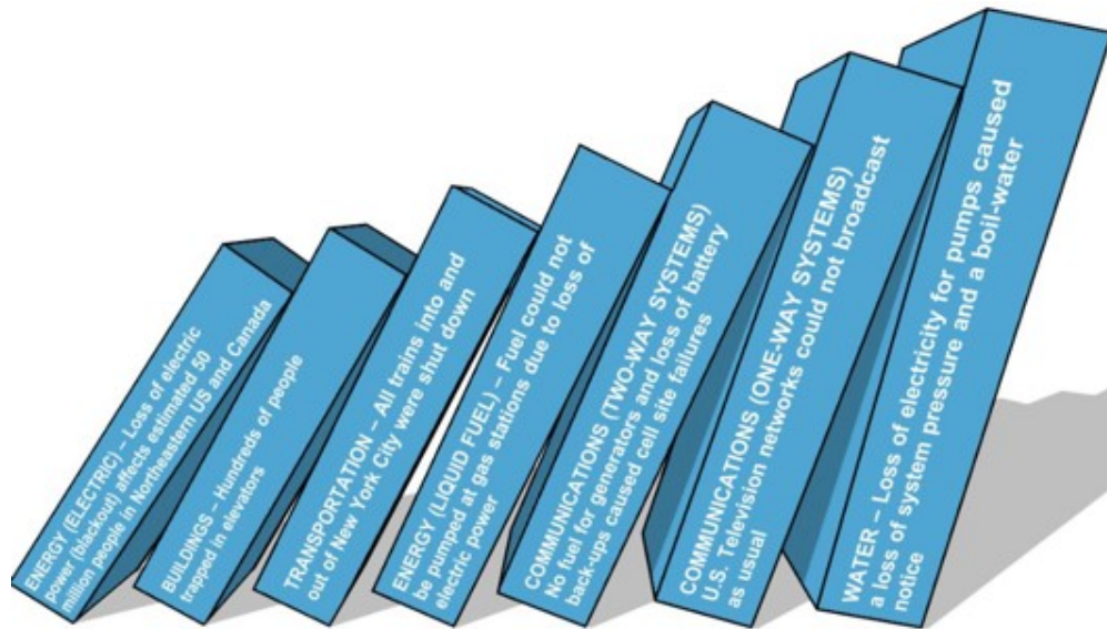
Figure 11-4: External dependence cascading failure in the 2003 Northeast Blackout
