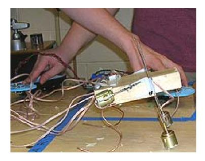
This is an uncovered 2-leg robot. It has two skids for support, and is being operated manually. The motors operating each leg are energized by one Control Unit, and each Control Unit is operated by a different student. Since the students' coordination is essential for the successful operation of the robot, teamwork is vital.
