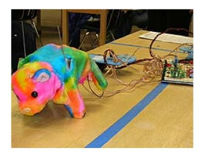
The picture (on the left) shows a finished 2-leg walking robot, which is operating in Automated mode. The Robot is about the size of a shoe box, and under the body covering is a block of wood with legs powered by 4 or more motors (see photo on next page).
