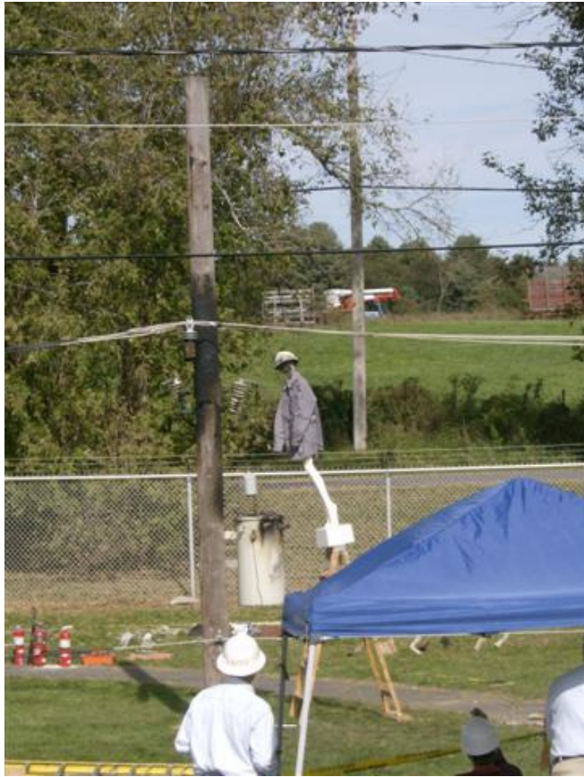
Figure 5 Arc Flash Demo utilizing a three-phase 4160 V distribution system, Full-scale mockup with mannequin "Joe the Lineman"
