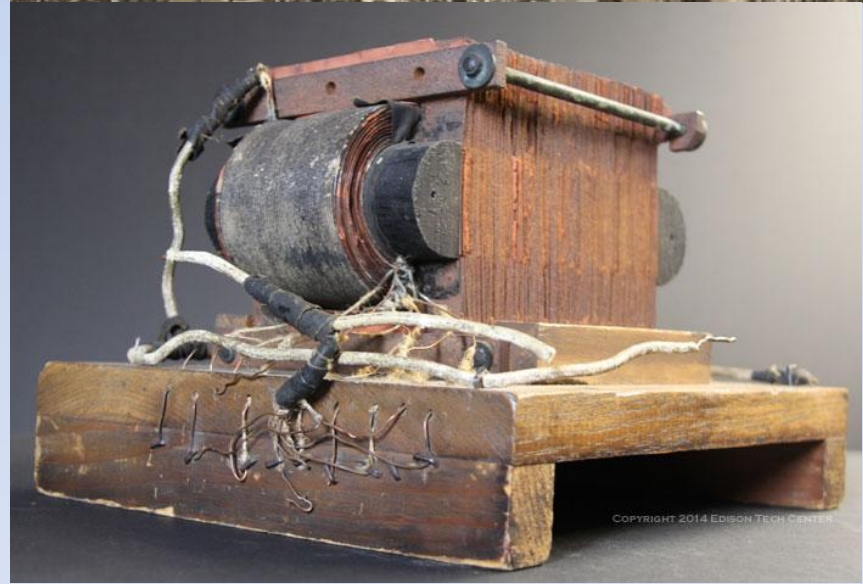
Great Barrington 1886 The first AC power distribution system using transformers (top) Stanley developed the prototype transformer (bottom) in 1885, it was robust, reliable and was a significant leap forward in technology.
