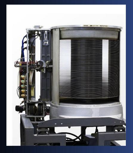
1950 – ATLAS stored data on the outside of a rotating cylinder. Utilized Ferromagnetic Materials and fixed read/write heads.
