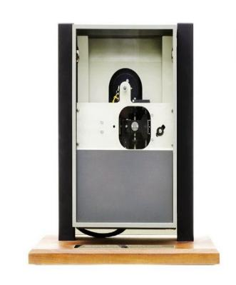
1962 – IBM 1311 Disk Drive was the first removable data storage device.
