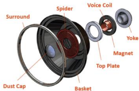
Image: Traditional Conical Speaker Driver Simplified Structure
