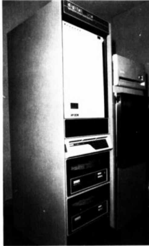
FIGURE 2.36 An overall view of an FPS AP-120B installation. The AP-120B occupies only 29 inches of rack space, and is attached to a PDP 11/34 with two disc units, a tape reader and output printer. The control teletype or VDU is not shown. (Photograph courtesy of D Head and Floating Point Systems, S A Ltd.)
