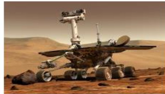
Figure 10. Spirit Rover on Martian Surface. Spirit is a rover that functions as a robotic geologist on Mars relaying mass amounts of critical data. Courtesy of NASA.
