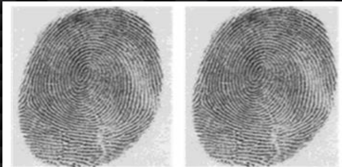
Figure 7 [1]. Comparison of Fingerprint Images. The one on the left is the original image and the one on the right is the wavelet compressed image (26 to 1 data compression).
