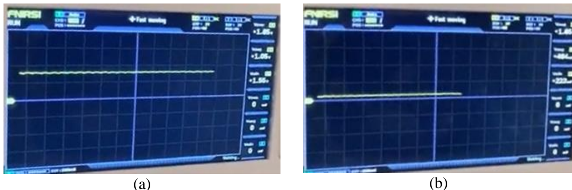
Figure 3.61 - (a) IR Sensor output with window blinds closed. (b) With blinds open.
