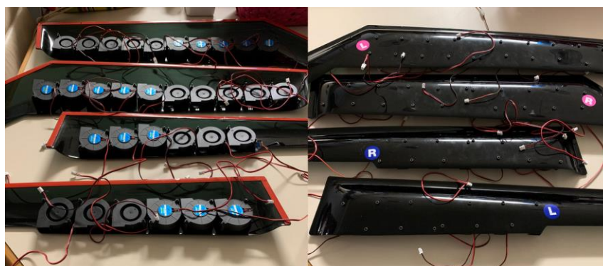
Figure 3.27 - Placement of DC Blowers on Vent Visors
