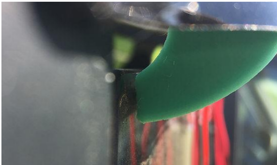
Figure 3.34 – First Revision Nozzle Minimal Clearance
