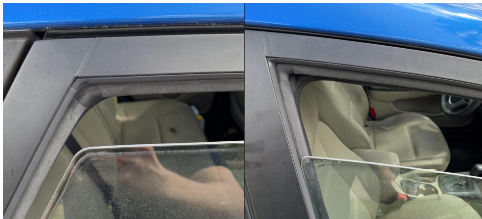
Figure 3.89 - Reference Vehicle Window Cracking
