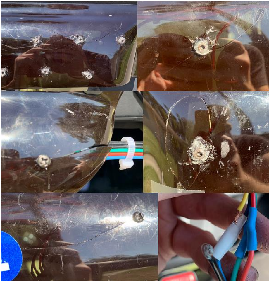
Figure 3.39 - Torque Damage Incurred by Vent Visors and Wire Break
