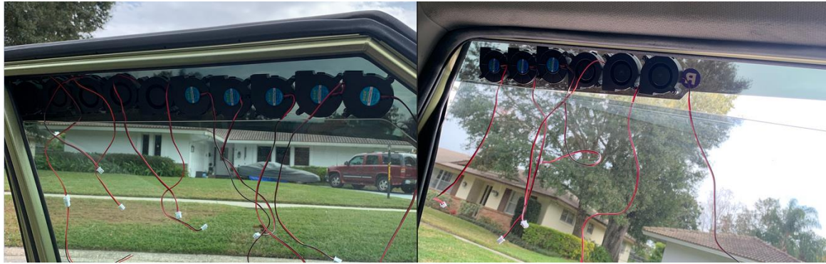
Figure 3.28 - DC Blower Array Attached to Car
