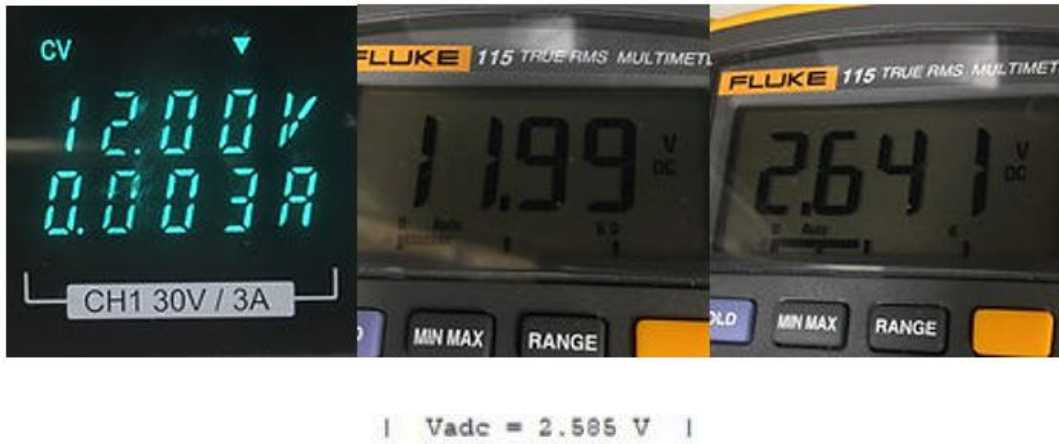
Figure 3.49 – ADC Voltage Test using DMM
