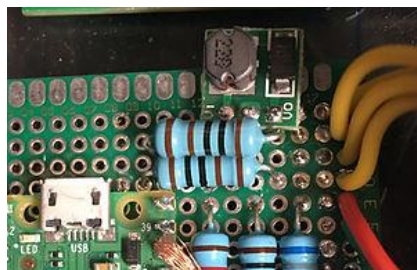
Figure 3.63 - Ultrasonic sensor components soldered to the MCU prototyping board
