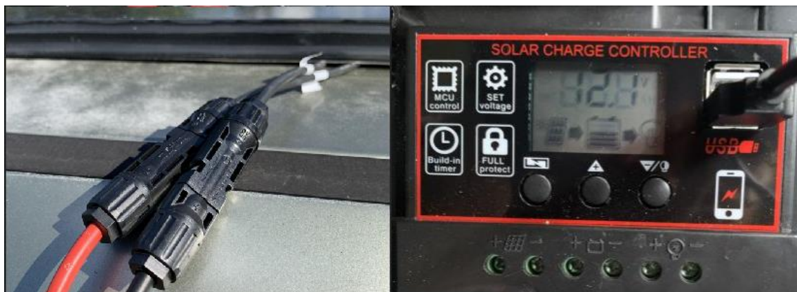
Figure 3.96 - PWM Voltage Post Re-connection of Solar Panel
