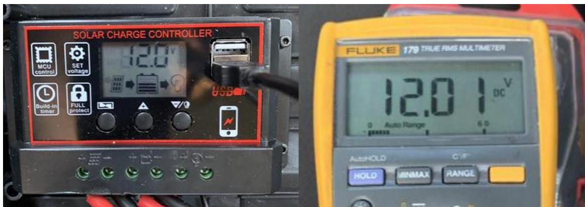
Figure 3.95 - PWM and DMM Voltage at Shutoff
