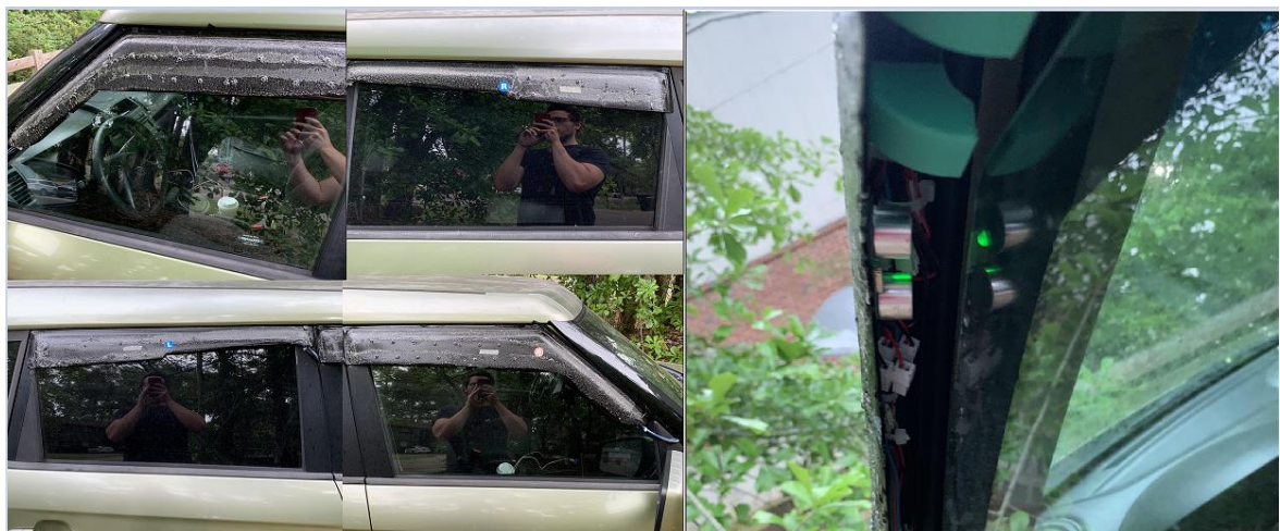
Figure 3.94 - Visual Inspection of Vent Visors and Activation of UUT
