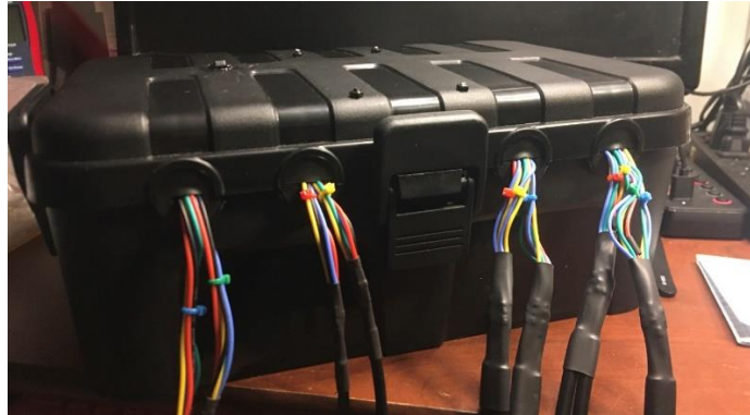
Figure 4 - Control module placed in control box
