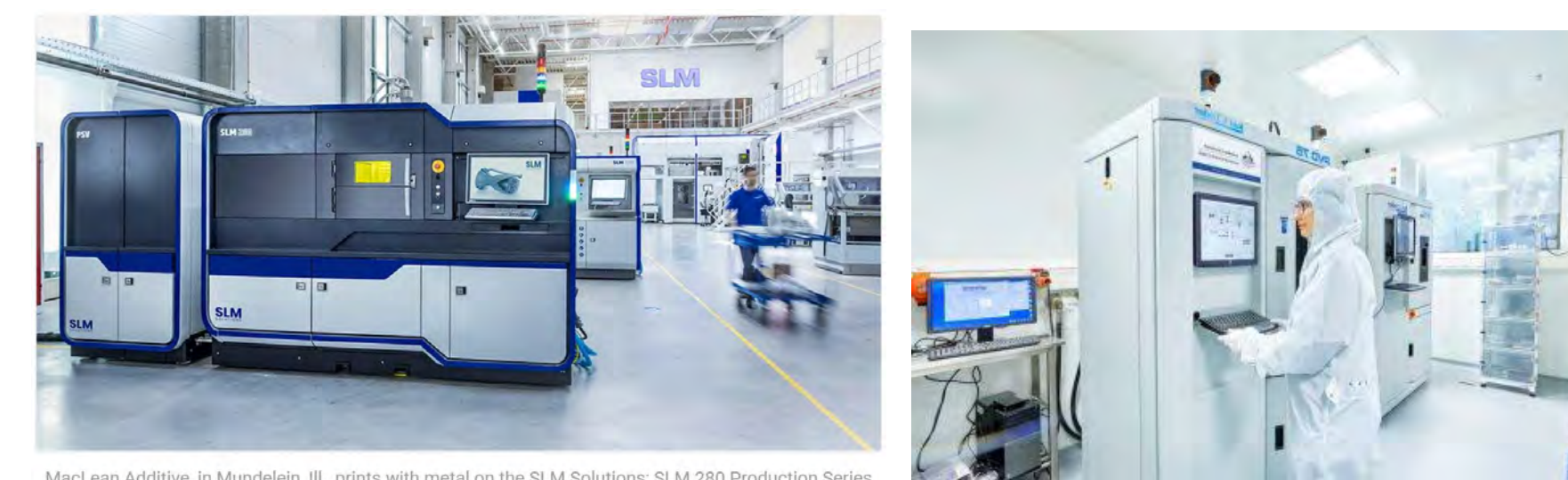
Fig 5: Conventional Metal Printer. 102" L, 48" W, 141" H - 4000 lbs
