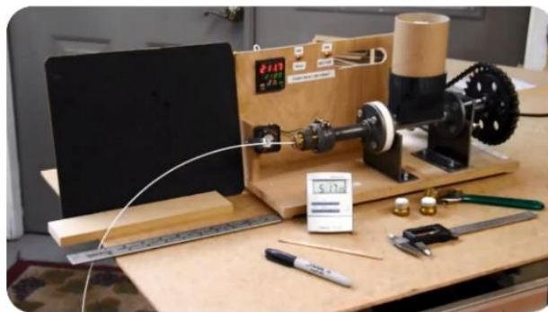
Figure 3. The customized Lyman extruder currently assembled in Dr. Barua’s lab at VCU is an open-source machine designed to turn polymer pellets into cheap filament for 3D printing.
