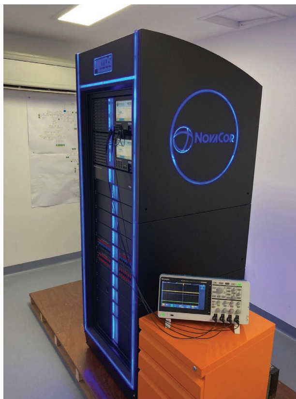
Figure 9. TasNetworks RTDS laboratory—NovaCor two rack (20-core) system.
