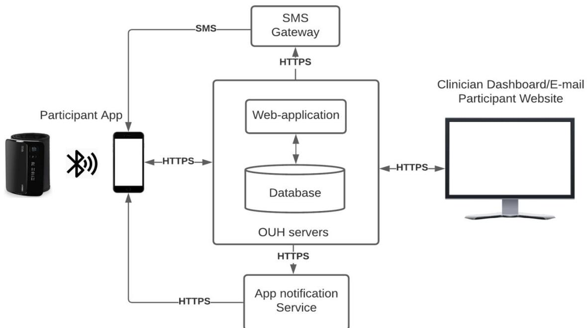
**Figure D.1:** Illustration of the POP-HT tele-monitoring system software and network architecture
