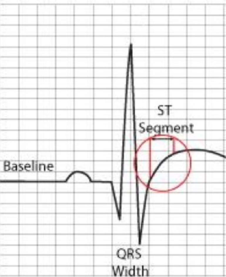
Figure 22: Possible' inferolateral STEMI: ST-segment shift
